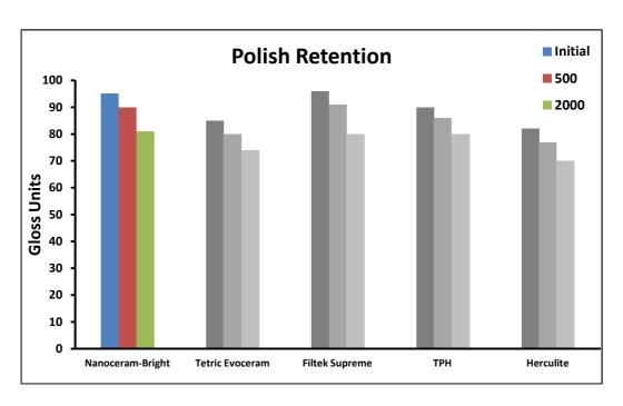
Figure 3: Polish retention of Nanoceram Bright versus other universal restorative materials
