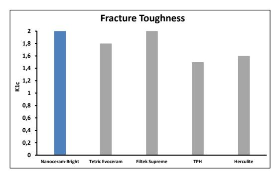
Figure 8: Fracture toughness comparison
