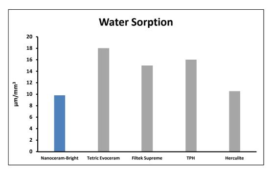
Figure 7: Water sorption comparison
