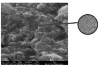
Figure 1: Nanoparticles evenly dispersed within the matrix
