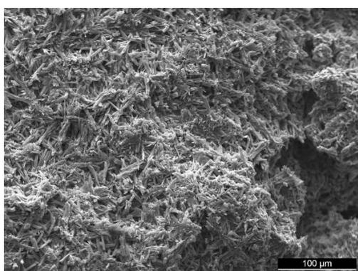
Figure 2: Post-setting structure, composed of needle like crystals, SEM
